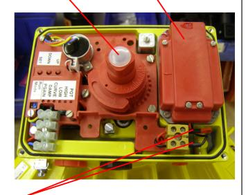
Measure the voltage across the contacts at 20mA you should get approximately 4.8 volts and the shaft should move.
