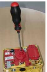
Lift out the carrier plate with the shaft.
