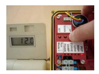
Press the SET and UP buttons: the LED flashes while the actuator's vane moves toward its 100% end stop. When its movement is stopped by the physical end stop, the positioner waits briefly, then moves the actuator steadily downscale until it runs against the bottom physical end stop, where again it waits briefly, and finally moves quickly back to the original position.
