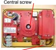
Servo valve wires / terminal block
