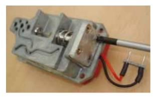
Replace the complete servo valve in its recess in the positioner body, taking care that the cork gasket under the servo valve rim is in place, fit the 4 screws with Loctite, screw them all down finger tight, and then tighten them down hard.
