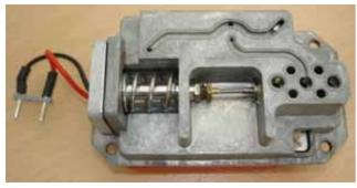
Observe the rubber gasket at the bottom of the frame and check whether it is clean. If not, replace it or clean it with ethanol and clean rag.
