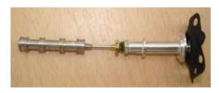
Clean the valve liner sleeve (in situ in the servo valve block) and the bobbin valve, using plenty of ethanol. Clean out the air channels as far as they are visible.
