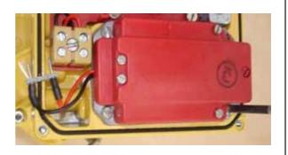
The complete unit can now be tested with 4-20mA signal.
