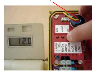
If the 'POT' LED flashes it means that the feedback potentiometer is set correctly – go to section 1.6
