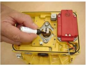
To replace the main circuit, first undo the 3 screws and remove the plastic cover. to expose the circuit.
