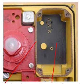
Top cork gasket Servo valve base gasket
